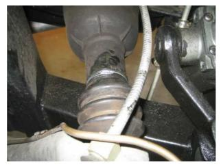
Make sure the two boot halves overlap and install a new wrap-wire on the outer rubber boot end to secure the two halves. Reinstall the brake drum, mount the tire, and readjust the brakes. Repeat the process on the other side and you're now ready for the road again!
