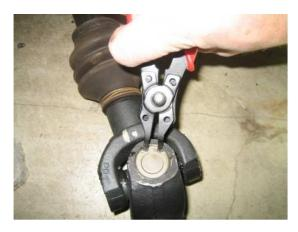
Using a pair of ring clip pliers, remove the two ring clips where the hub connects to the universal joint. Depending on when you last touched the universal joint, it may be easy to tap out the bearing cups or you may end up needing to press them out with a hydraulic press. I used a socket that was just slightly smaller than the cup diameter to tap out the universal joints. If they've been in there long enough to need a press, this may be a good opportunity to replace them with new ones.
