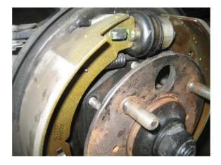
Next, pull the entire hub assembly out through the trailing arm. At this point you'll have the hub assembly with <sup>1</sup>/<sub>2</sub> the <sup>1</sup>/<sub>2</sub> shaft (I guess that makes it a quarter shaft ).
